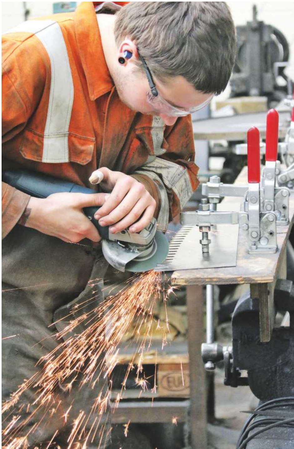
▲ Flinn apprentice Nathan hard at work sharpening a logging saw with a grinder
